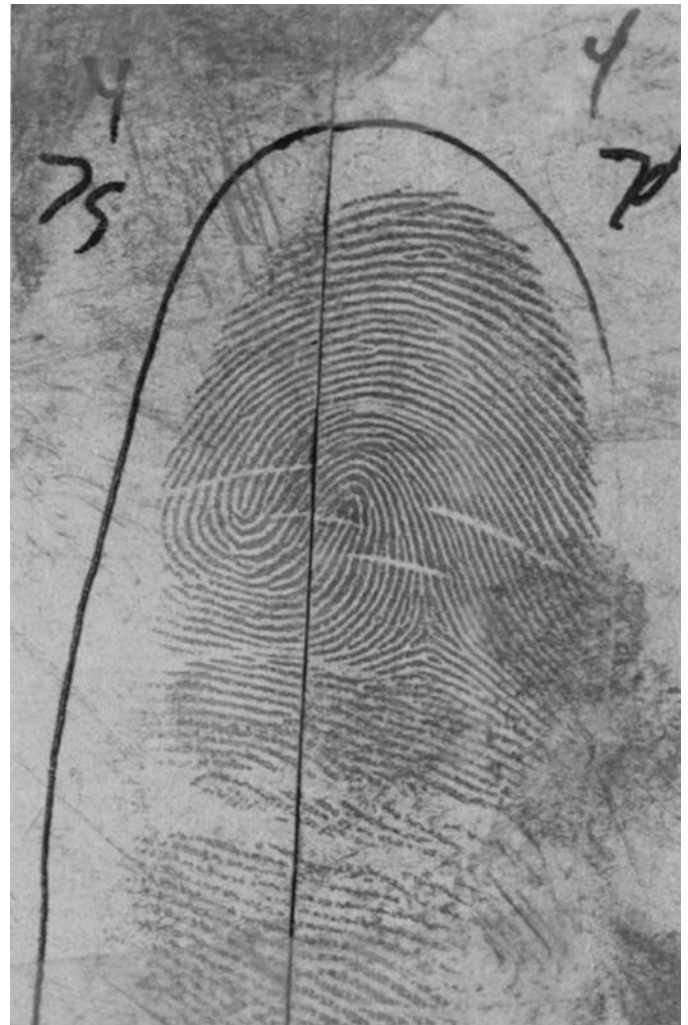
FIG. 6—Left side of print was developed with the new formulation made with 75 g ferrous ammonium sulfate hexahydrate. Right side of print was developed with the new formulation made with 70 g (right) ferrous ammonium sulfate hexahydrate.
