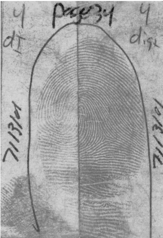
FIG. 1—Left side of print (labeled DI) was developed with the current formulation (with RO/DI water). Right side of print (labeled dist) was developed with current formulation (with distilled water).
