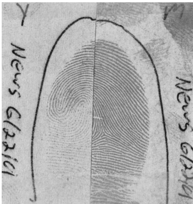
FIG. 7—Latent print placed on newspaper on 6/22/01 and processed on 7/10/02 with the current formulation (left) and with the new formulation (right). Both solutions were made on 7/3/02 (seven days old).
